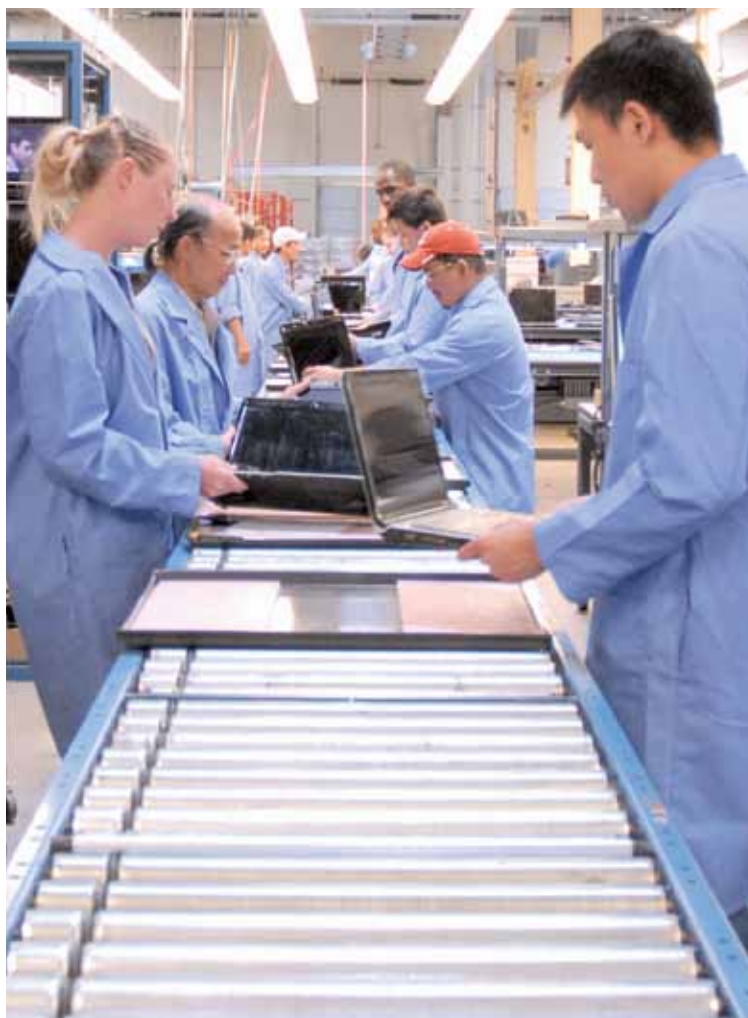
Image Microsystems technicians inspect returned electronic devices to determine whether the products should be repaired, resold, or scrapped.
